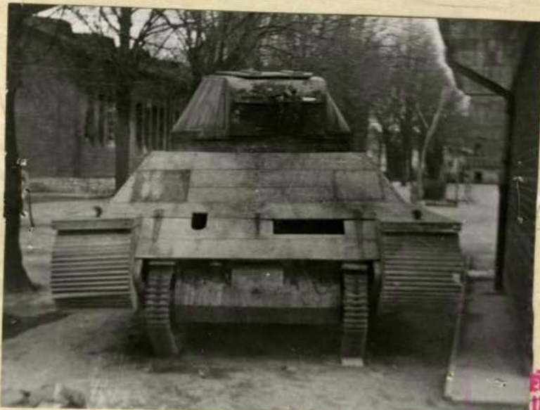
Photo No. 2 Front view. Note vision openings.
