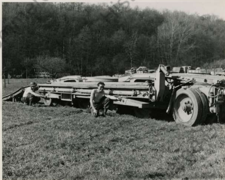
Photo No. 6 Right side of trailer showing suspension points of platform. Suspension points are shown as "b" in diagram, Appendix "A".
