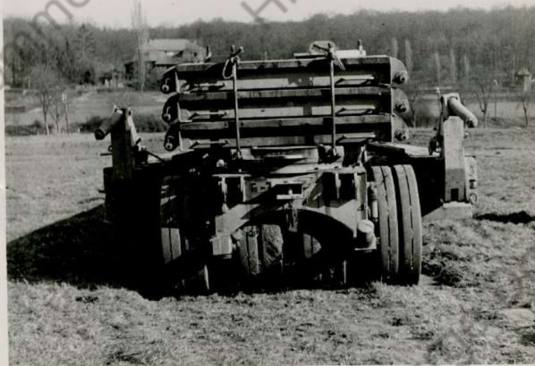
Photo No. 3 Front view showing ramp sections stowed and held in place by hold-down rods. Note holdfasts for securing loaded tank on each side.
