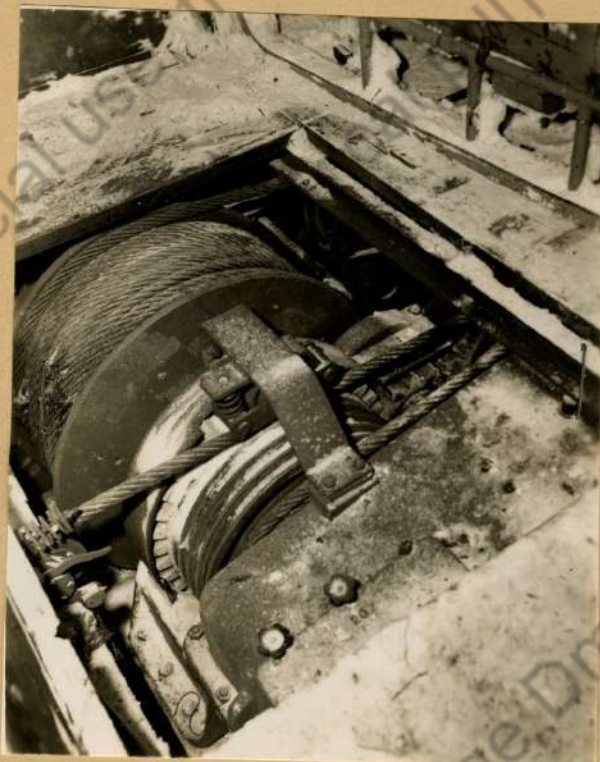
Photo No. 3 Rear half of winch showing part of gear case, rear power pulley and cable drum. Guide roller is mounted over power pulley.
